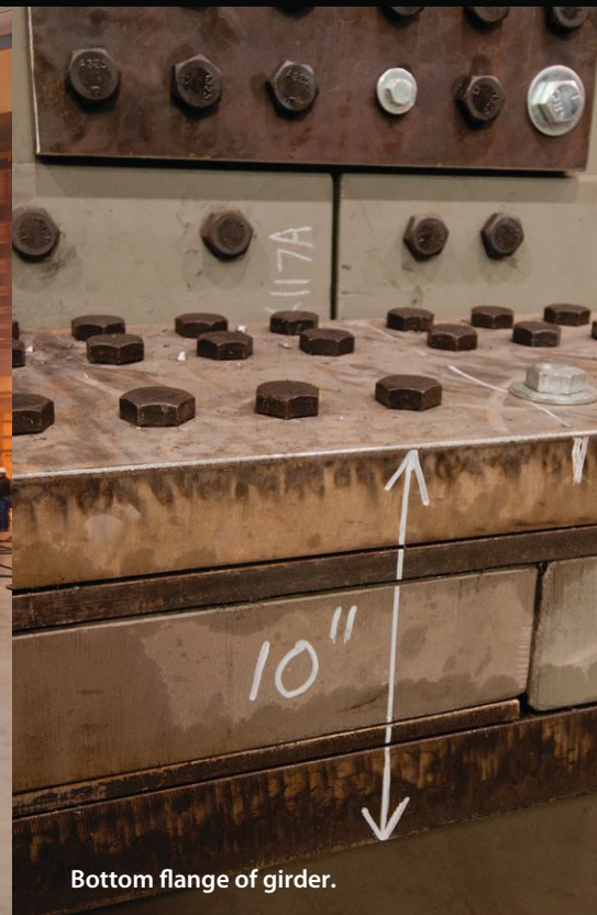
80-foot long railroad girder with bolt holes drilled zero to 80 feet within 1/32-inch.
